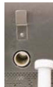
Ceramic tube port for thermocouples during temperature survey. When not in use, an insulating plug is supplied.
