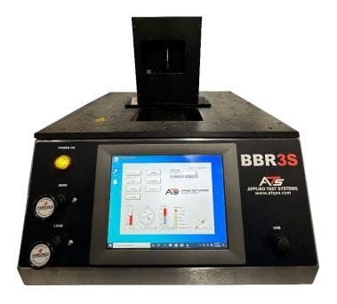
The ATS Bending Beam Rheometer 3S (BBR3S) performs flexural tests on asphalt/bitumen binder and similar specimens per AASHTO T 313, AASHTO TP 87, ASTM D6648, GOST 58400.8-2019, and BS EN 14771 specifications as part of the PG grading system according to Superpave. An ATS original, the BBR3 is the first of its kind to offer a state of the art internal computer system, incorporating intuitive new software and touchscreen technology.
