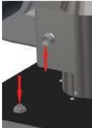
Figure D.2: Draft inducer tubing must be installed here for proper operation
