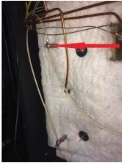
Figure H.7: Heating element connections (4) & insulation retainers
