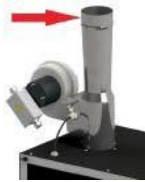
Figure D.4: Attach a 6"-8" section of flexible duct to the 4" OD Draft Inducer Outlet using a 4"-6" transition adapter.
