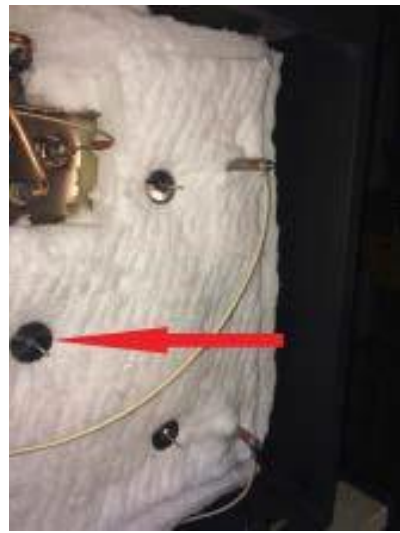
Figure H.8: Heating element connections & insulation retainers (5)
