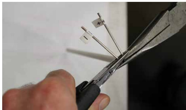
Figure G.7 - Bending Thermocouple Wires
