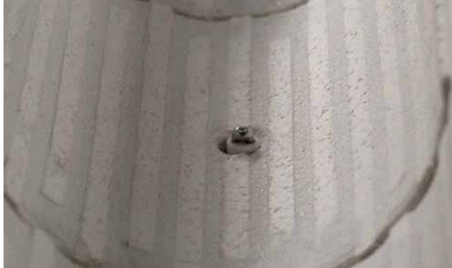
Figure G.8 - Thermocouple Extending Past Element
